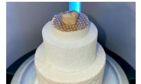
The crown is placed on top of the CEREC SpeedFire honeycomb tray with a firing pad. It must be centered on the pad. The construction is then placed in CEREC SpeedFire.
