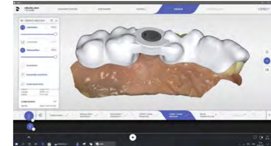
After importing the implant and sleeve planning, the CEREC Guide 3 drill template is designed using CEREC Software.
