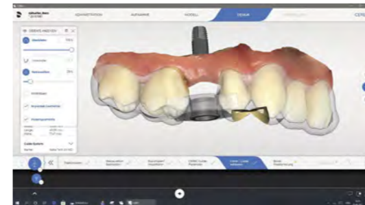
Semi-transparent representation of the CEREC Guide 3 drill template. The metal sleeve is shown, which is glued into the perforation after milling the surgical template.
