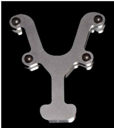
Figure 1. Metallic reference aid with four steel spheres.
