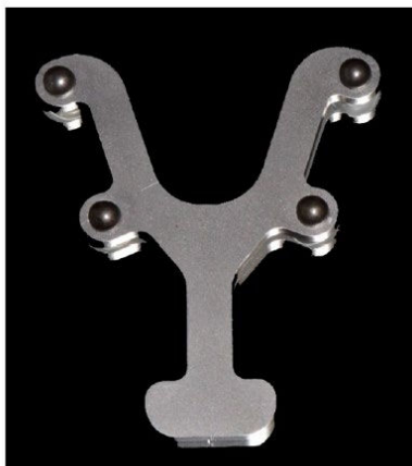
Figure 1. Metallic reference aid with four steel spheres.
