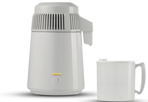
Water distiller for obtaining distilled water by boiling and subsequent steam condensation. It distils 0.7 L of water per hour. 4-litre capacity. It fulfils the safety and electromagnetic compatibility (2014/30/EU) and low voltage (2014/35/EU) tests.
