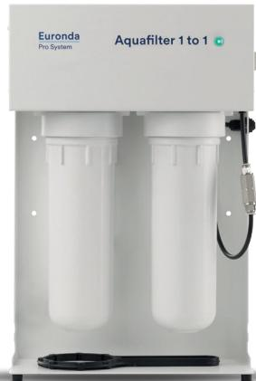
Device for the production of deionised water for autoclaves, in accordance with EN 13060 (< 15 µS/cm). Only one Euronda Pro System autoclave can be supplied. It deionises on average 1 litre of water per minute. It can be equipped with automatic shut-off device. It can be placed directly on the worktop or inside a cabinet, as well as mounted to a wall. Included in the initial equipment are two ion exchange resins.
